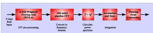
**Fig 2** Block diagram of the FPGA signal processing pipeline
