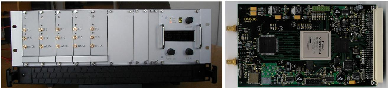
**Fig 4** Prototype of the MPIfR broad-band Array FFTS (AFFTS) equipped with 5 FFTS boards (right). The final AFFTS will consist of four crates with 8 FFTS boards each. A single board will provide 1.5 GHz bandwidth with 8K channels.
