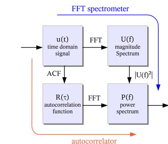
**Fig 1** "Wiener-Khinchin-Theorem": FFT spectrometer implement an alternative approach for obtaining the power spectrum of a given time signal.
