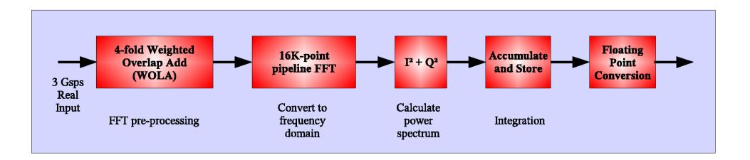
Fig 2 Block diagram of the FPGA signal processing pipeline
