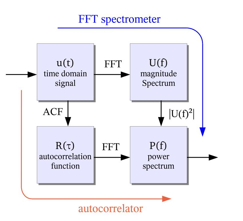
**Fig 1** "Wiener-Khinchin-Theorem": FFT spectrometer implement an alternative approach for obtaining the
