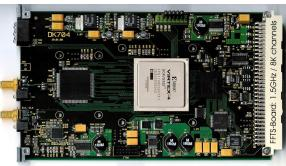
The MPIfR Array-FFTS, now operated at APEX, is equipped with 8 FFTS boards and the FFTS controller. A single FFTS board provides 1.5 GHz instantaneous bandwidth with 8192 spectral channels. The frequency resolution (equivalent noise bandwidth) in this standard configuration is 212 kHz.
