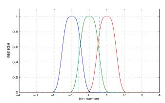
Frequency response of the optimized FFT signal processing pipeline. The dashed lines illustrates the equivalent noise bandwidth (ENBW) for the corresponding spectral bin.
